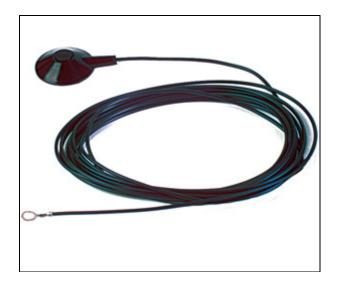
Use the cord to connect all Electrically Static Dissipative floor mats to a building ground. The solderless terminal can be connected to an electrical outlet using the screw in the outlet cover.
